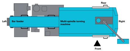
Illustration 2: Physical locations of a multi-spindle turning machine, example
