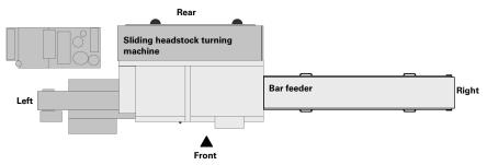
Illustration 3: Physical locations of a sliding headstock turning machine, example
