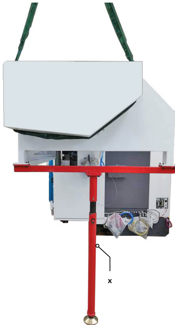
Fig.: Crane support during assembly/disassembly of support leg (x) WHU (height-adjustable)
