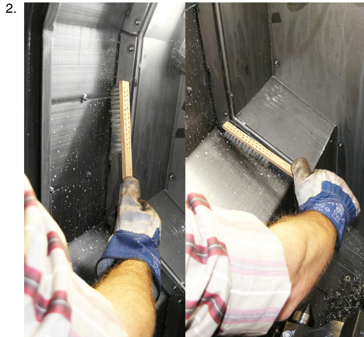
Example: 2 Sweep small chips and other debris from top to bottom using chip brooms or brushes.
