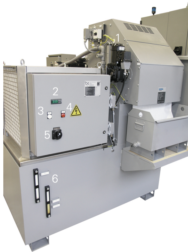
Example: Cooling lubricant reconditioning R200
