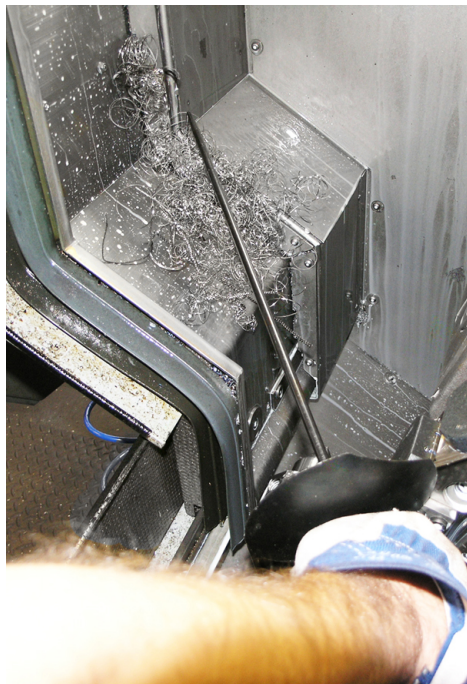
Example: 1 Removing chip nest using appropriate tools (e.g., chip hooks)
