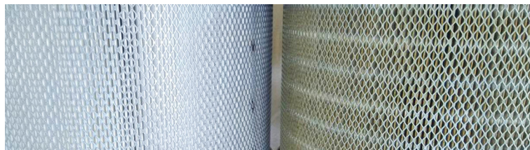
Post-filter for cutting oil mist: left new – right used
