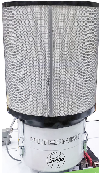
Post-filter for cutting oil mist
