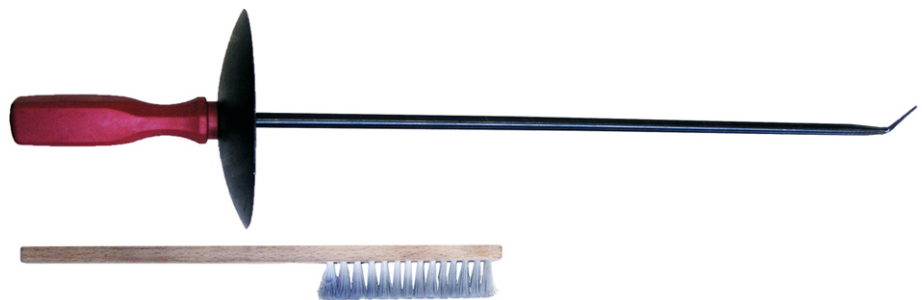
Example: Chip hook and chip brush
