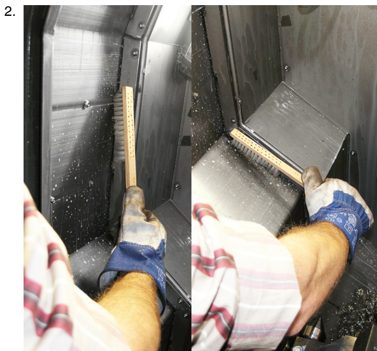
Example: 2 Sweep small chips and other debris from top to bottom using chip brooms or brushes.
