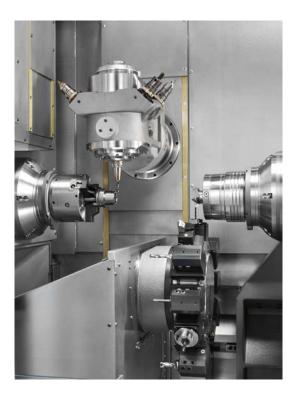
Figure 3: Tool turret: Is available with 18 or 12 stations and has a Y-axis with a traversing range of +/-50 mm.
