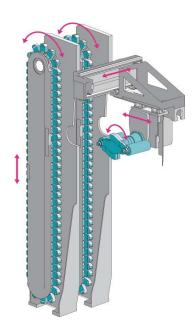
**Figure 5:**Tool magazine: Large tool magazine with up to 140 stations (HSK-T40), designed with double rows
