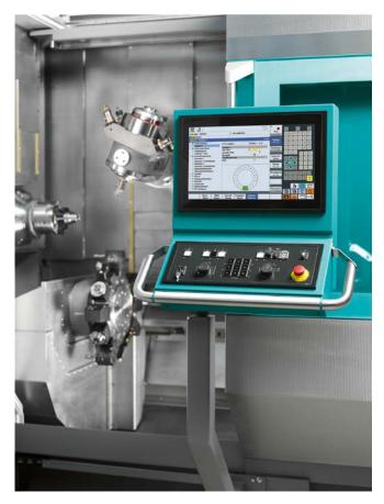
**Figure 6:**Operation: The latest INDEX C200 sl control generation, based on the Siemens Sinumerik 840D sl (solution line) and an 18.5" touch-sensitive wide-screen monitor.
