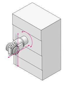
During development of the R series, emphasis was placed on achieving a high degree of stiffness, thermal and dynamic stability, and vibration damping. For this reason, a vertical cast machine bed with a heavily ribbed, enclosed modular design was chosen. The motorized milling spindles are placed in the center of the machine and are operated freely and wearfree in the Y- and B-axes via hydrostatic circular guides. The guide system contributes considerably to the
