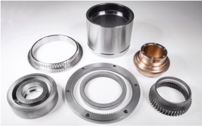
Power skiving on the INDEX G220 turn-mill center: This process combines cutting and rolling operations in which the tool and workpiece rotate synchronously. The ring gear for a three-stage planetary gear features one helical and one spur internal gear profile, as well as an external knurled geometry for press-fitting into the housing. All three profiles are produced by power skiving. Photos of the workpieces: Framo Morat
