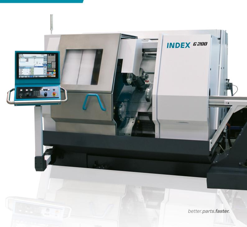
Take advantage of the option to increase the performance and flexibility of your machine. Refit your INDEX G200 with the latest SIEMENS controller and benefit from a wide range of improvements. After the refit, your machine can be connected to the iX4.0 IoT platform, making you ideally equipped for the digitization of your production environment
